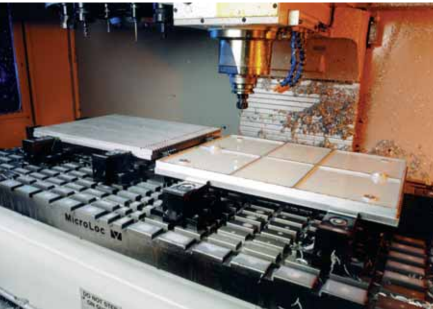
Matched pairs of escalator treads being machined at Finecast Engineering Ltd
