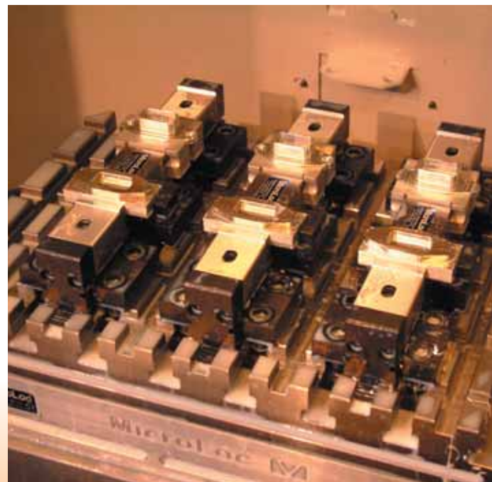
50-series system machining aluminium parts for the electronics industry on a Brother machining centre
