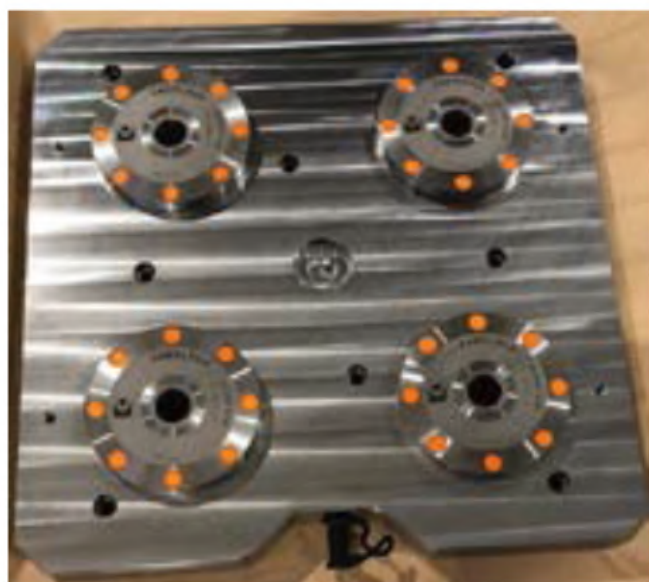
4 EASYLOCK zero point Unit Base
